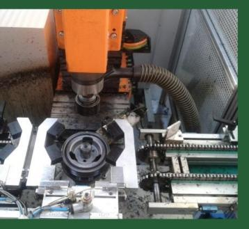
Rotation of the pulley according to a mark + Measurement of the unbalance Removal of material
