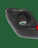
When the edge of a plate is worn, put a shot of red paint.
